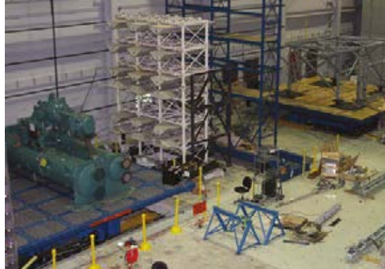
SEESL's twin relocatable shake tables
