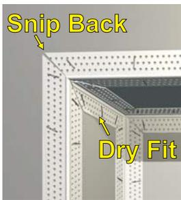
**Step 2:** On vertical corners, do not allow the bead or bulladapter to touch the floor. Always install with a 1/2" gap to prevent structural settling from cracking the mud. If you're using 2 ways, 3 ways or Bulladapters install these first with 847 Spray Adhesive & Staples. To glue the bead to the molded corners, put a dab of adhesive caulk on the tabs of the corners. Where beads meet, snip back mud legs as shown. Do not overlap mud legs. Dry fit as needed.
