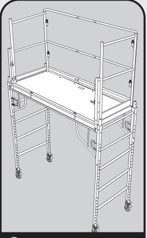
Once hinges are fastened, close end panel and secure with latch. Once guardrail system is installed and secured to multifunction unit, tighten fender screws at toe board connector to complete the guardrail system.
